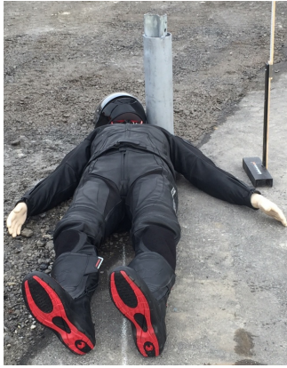
Figure 4: Biofidelic crash test dummy at impact point ( sigma post covered with a pipe )
